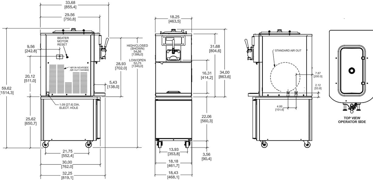
NOTE: FIGURES IN BRACKETS INDICATE MILLIMETERS / DECIMAL AND FRACTIONAL DIMENSIONS EQUAL TO ( PLUS OR MINUS 1/16 INCH [1.5mm] ).
